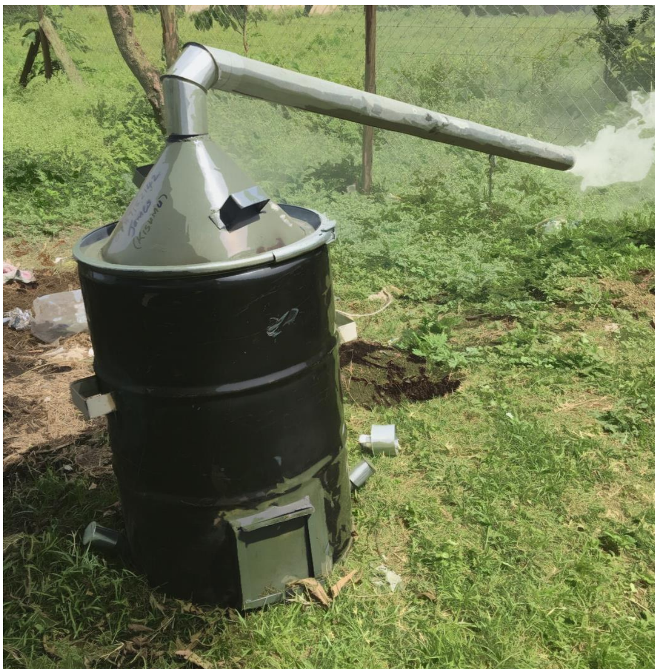
Figure 2-3: Carbonisation equipment made from used oil barrel. Photo Credit: James K. Gitau
