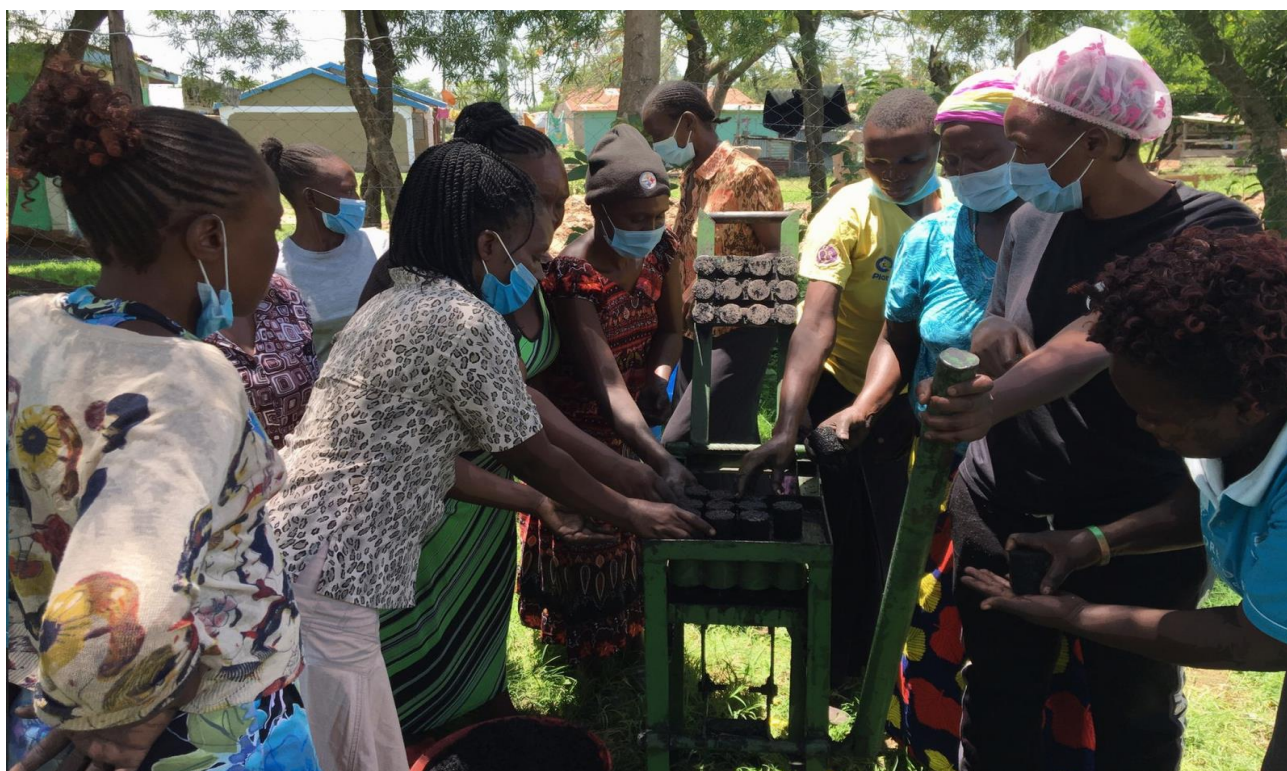
Figure 2-7: Women compacting briquette using a manual briquetting machine. Photo Credit: James K. Gitau
