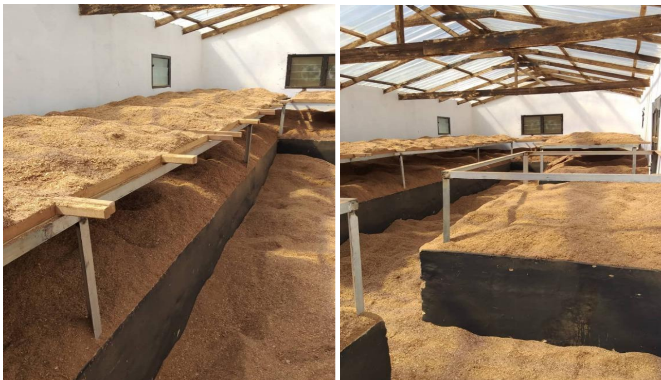
Figure 2-2: Sawdust is passively dried in a solar dryer at Somanya Biomass Briquetting Plant in Accra Ghana. Photo Credit: Dzifa Agbefe, IWMI
