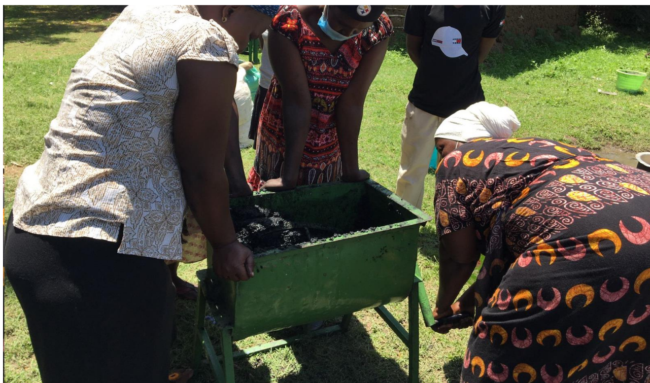
Figure 2-6: Women mixing carbon dust and binder using a manual mixer. Photo Credit: James K. Gitau
