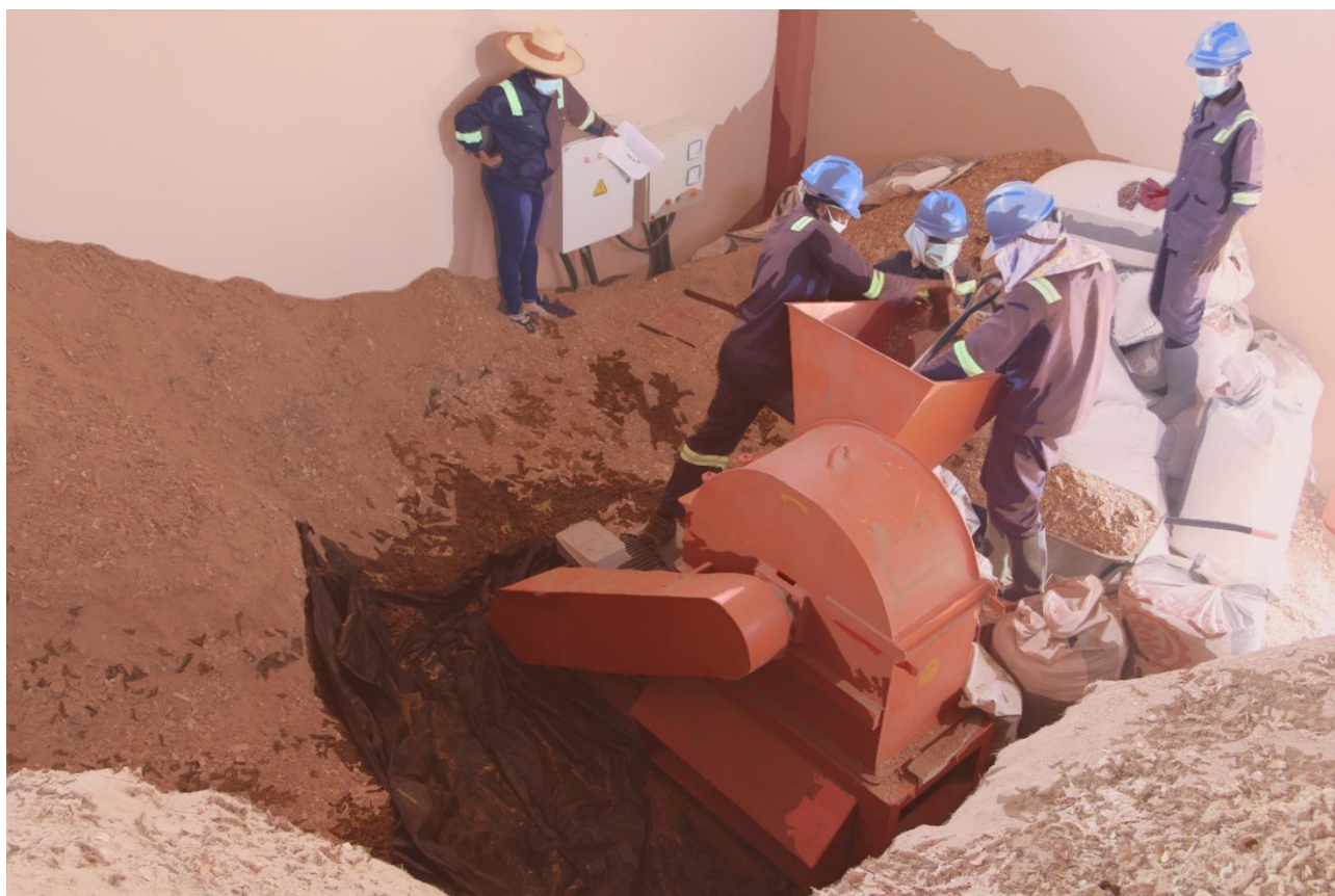
Figure 2-5: A mechanical crusher in Somanya Plant used for wood chips. Photo credit: Dzifa Agbefe, IWMI
