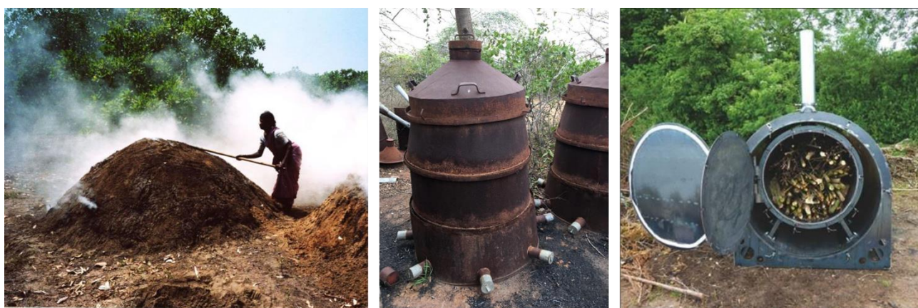
Figure 2-4: Examples of different carbonisation equipment. a) wood charcoal production with a traditional earth mound kiln near Pondicherry, India, b) a burn kiln made from used oil barrels in Kenya, c) Retort kiln design based on two-chamber, the inner cylinder filled with wood (as cited in Uwase et al. 2022). Photo credits: Adam, 2004 as cited in Biocoal.org (Left), James K Gitau (Middle), Uwase et al. 2022 (Right)
