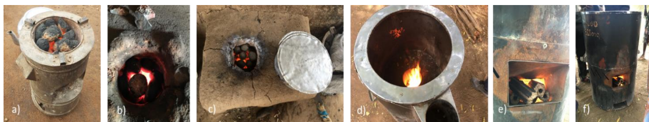
Figure 2-8: Cooking with carbonized briquettes in a domestic cookstove (a-c) and institutional stove (d-f) Photo credits: James K. Gitau
