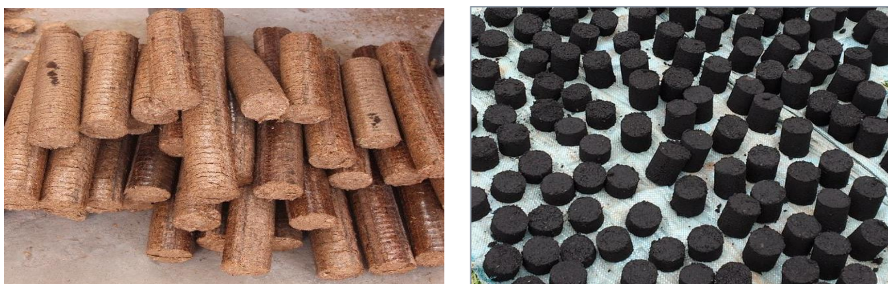
Figure 1-1: Sample of non-carbonised briquettes made with a briquetting machine (left) and carbonised briquettes moulded by hand (right). Photo Credits: James K Gitau (right); Dzifa Agbefu, IWMI (left)
